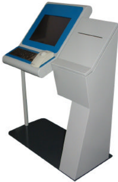
REACH kiosk shown with keyboard, 17.1" TFT Touch monitor & thermal roll printer option.
